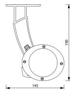
**Example – One Electric Dimensions** Model: OE240 Screen width: 2400mm Total width: 2400 mm + 78 mm = 2478 mm Bar width: 2400 mm + 11 mm = 2411 mm
